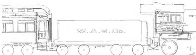
Fig. 2422. Diagram of Westinghouse Train Air Signal Equipment.
